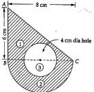
(b) Determine the centroid of the wire shown in below figure.
